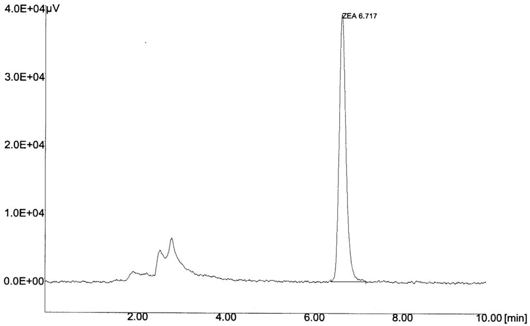
Figure 6: Sample chromatogram of a corn sample spiked at a level of 250 µg/kg
