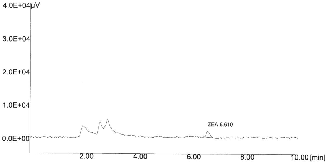
Figure 5: Sample chromatogram of a corn sample spiked at a level of 10 µg/kg
