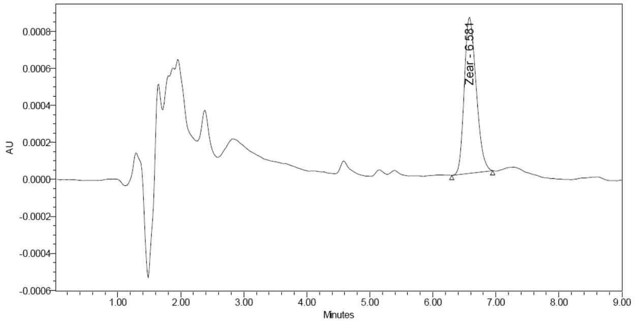
Figure 4: 200 ppb recovery of spiked corn with absorbance detector
