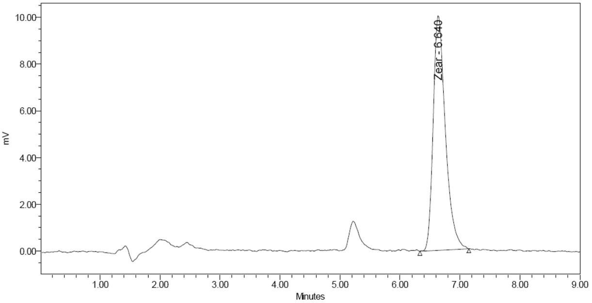
Figure 2: 250 ppb recovery of spiked corn with fluorescence detector
