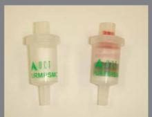
Comparison of mini-cartridges before (left) and after (right) cleanup of 1 mL red wine extract
