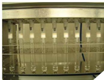
Photograph of FAST® set-up using a positive pressure manifold system. The beverage samples were passed through the FAST® cartridges, with unwanted matrix components retained onto the sorbents (yellowish color), while the cleaned samples were collected in the test tubes
