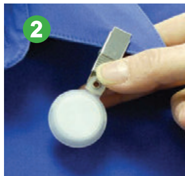
Clip in worker's breathing zone to sample.
