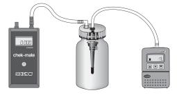
Figure 3. Calibration Train with Jar
