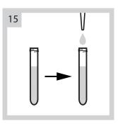
Use pipette to transfer 2 ml prepared sample to a new Total N - LR or Total N - HR vial.
