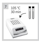
Put the vials into CR 25 reactor then start to countdown from 30 mins at 105°C.
