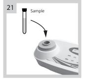
Insert the test sample vial into WD 100 colorimeter to start a test.
