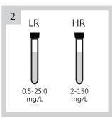
Select the appropriate concentration of reagent according to the nitrogen concentration of sample.
