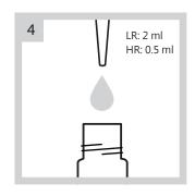
Add pure water to one reagent vial as the blank sample. Adding volume is as below: LR: 2 ml, HR: 0.5 ml.
