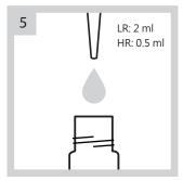
Add sample to another reagent vial as the test sample. Adding volume is as below: LR: 2 ml, HR: 0.5 ml.
