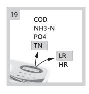
Turn on WD 100 colorimeter, then select test item and concentration range.
