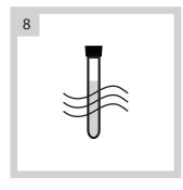
**Immediately** remove the vials at exactly 30 mins and cool vials down to room temperature.
