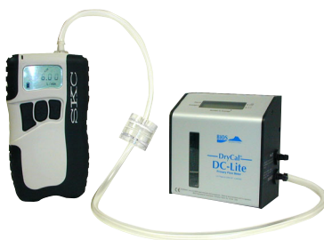
Calibration train with sample medium in-line
