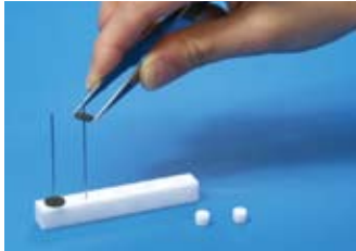
MT Holder & MT Stand Grasp the MonoTrap™ with tweezers and insert the holder into the hole of the MonoTrap™.
