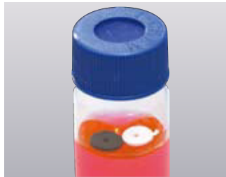
Put the sample into the vial and add MonoTrap
