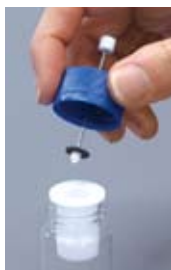
Insert the MonoTrap and tighten the septum
