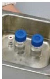
Give it ultrasonic agitation for 5 mins
