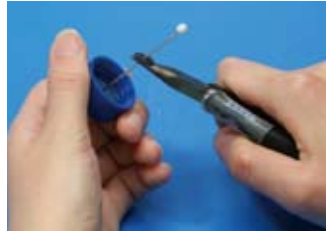
Hold MT Holder with pliers whose ends have been cleaned and pass it through the septum. Put a cap on top of the holder.
