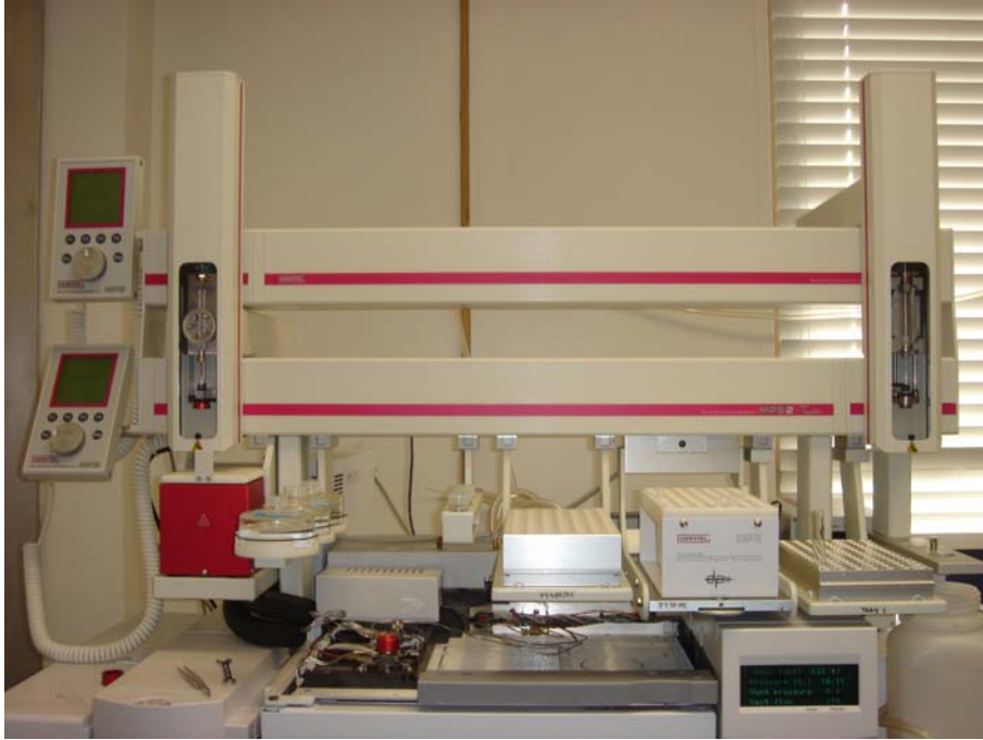
Figure 2. A picture of the dual rail MPS-2 system, which stands on top of the GC/MS system. The left syringe performs large volume injections, and the right syringe performs automated DPX extractions.
