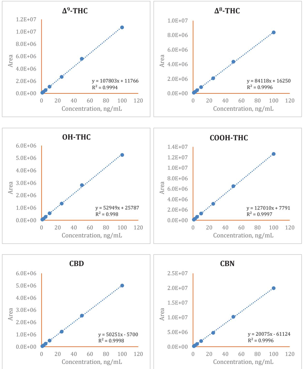
Figure 3. 7-point neat calibration curve for all analytes with linear equation and R<sup>2</sup> value.
