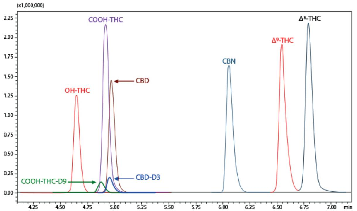
Figure 1. Chromatogram of extracted 50 ng/mL blood sample
