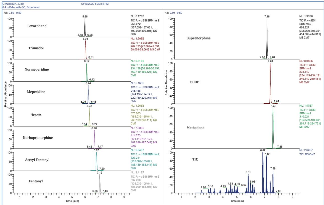
**Figure 1:** Exemplary chromatogram of the separation obtained using the Selectra® DA UHPLC column. All analytes included in the method eluted in less than 8 minutes. The TIC represents the total ion chromatogram for a single injection.
