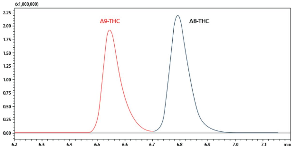
Figure 2. Zoomed in chromatogram of 50 ng/mL extracted blood sample showing separation of THC isomers
