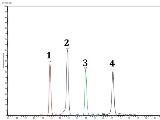
**Figure 2a:** Complete separation of critical isobaric compounds 1) Morphine, 2) Hydromorphone, 3) Norcodeine, and 4) Norhydrocodone.
