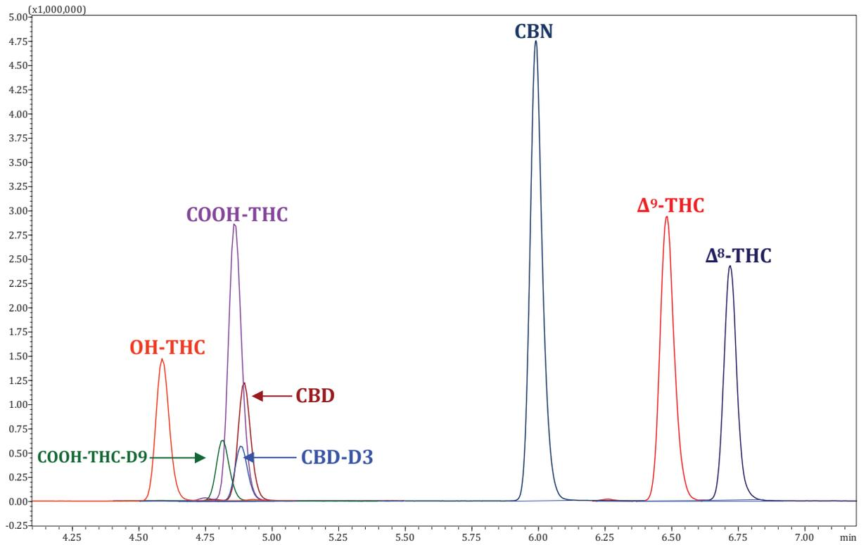
Figure 1. Chromatogram of extracted 50 ng/mL urine sample, minutes 4.10 – 7.20
