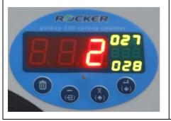
After releasing the "EXIT" key, the saved counts will display on LED-B/C/D. The selected count will flash and LED-A will show the record number of selected count.
