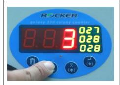
After finish counting, press and hold "EXIT" key for 1 second to enter < View Mode > to check the saved counts.
