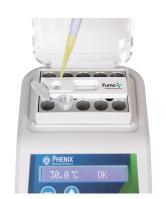
Insert the Fumo-V strip into the Vertu. Press the center key to take a reading. To print, use the arrow keys to move the cursor to "P" and press the center button.
