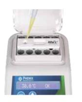
Insert the Afla-V strip into the Vertu. Press the center key to take a reading. To print, use the arrow keys to move the cursor to "P" and press the center button.
