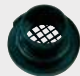
Conductive plastic cassette for gravimetric determinations
