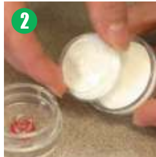
Weigh Accu-CAP and insert in cassette.
