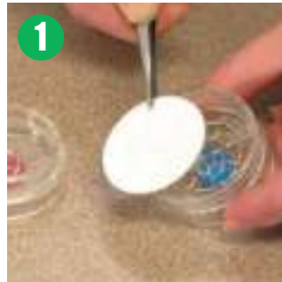
Prepare SKC 2-piece cassette with support pad.
