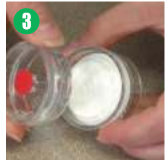
Complete cassette assembly. After sampling, remove Accu-CAP from cassette and weigh.
