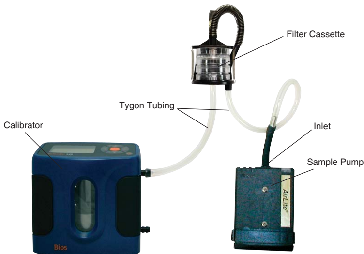
Calibration train with filter cassette
