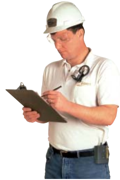
Clip sampling medium to worker and pump to belt.
