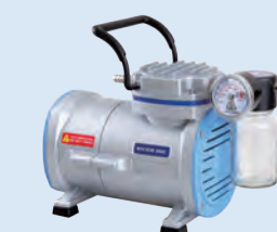
Rocker 300C Max. vacuum : 99 mbar abs. Max. flow rate : 23 (20) L/min
