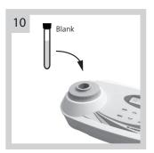
Insert the blank sample vial into WD 100 colorimeter to start a zero calibration.
