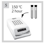
Put vials into CR 25, COD reactor then start COD program to heat at 150°C for 2 hours.
