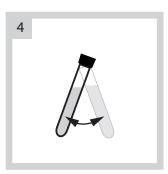
Tighten the vial cap and shake slightly to mix evenly.
