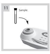
Insert the test sample vial into WD 100 colorimeter to start a test.
