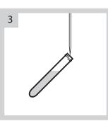
Hold vial at 45-degree angle. Add 2 ml sample to another COD reagent vial as the test sample.
