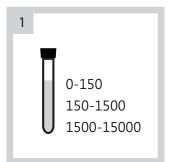
Select the appropriate concentration of reagent according to the COD concentration of sample.
