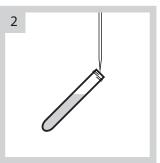
Hold vial at 45-degree angle. Add 2 ml pure water to one COD reagent vial as the blank sample.
