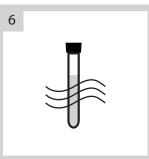
Turn off CR 25 reactor after digestion and wait vials to cool to room temperature.
