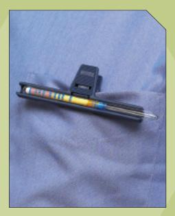
Figure 3 Note the end of the color change and record your reading. Then, simply divide by the number of hours for the TWA (PPM hours/hours worked).
